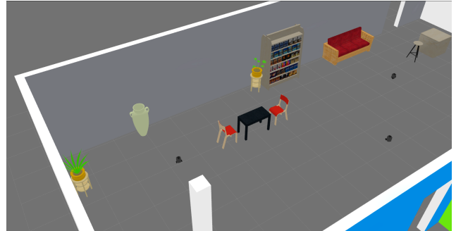
Fig. 1. Gazebo simulation of 3 Turtlebot3 robots in house environment. Our simulator accounts for realistic physical constraints such as communication delays, line-of-sight limitations, and computational constraints, and implements processes for sensing, map reconstruction, and coordination with reduced resource requirements.
